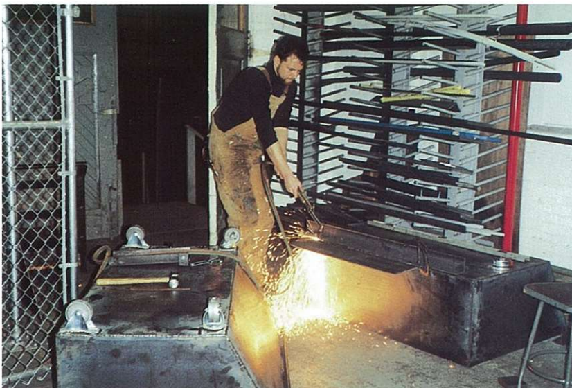
New steel dump carts with wheels being fabricated.
