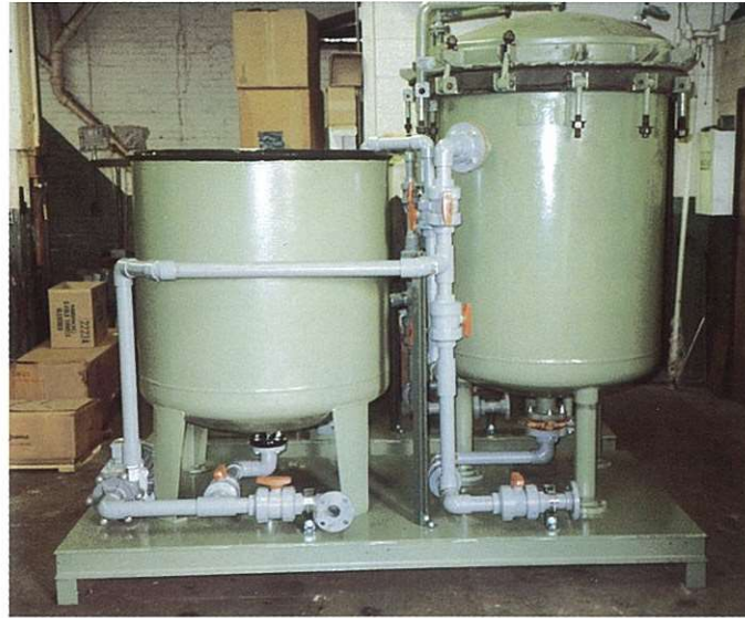
5000 gallon per hour horizontal plate nickel plating filter that was rebuilt by Met-Chem. The rebuild on this particular unit included:
