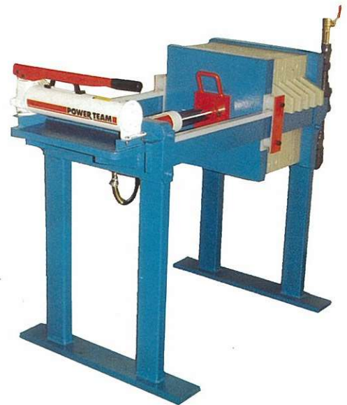
1 cu. ft. 470mm filter press with manual closure. Unit closes hydraulically and opens with spring assisted return, pulling follower plate with it.
