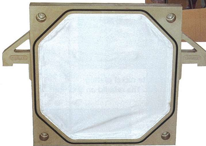
Replacement filter press cloth installed in a plate.
